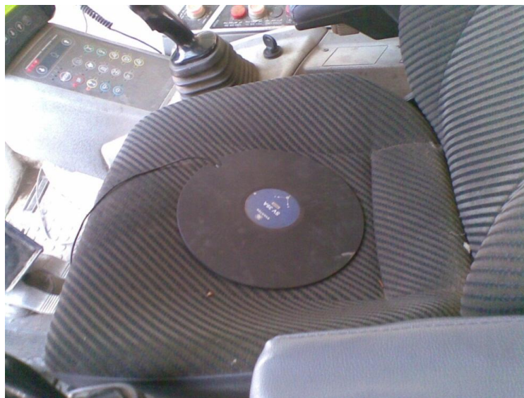
Figure 1: Position of vibrometer sensors on the seat
