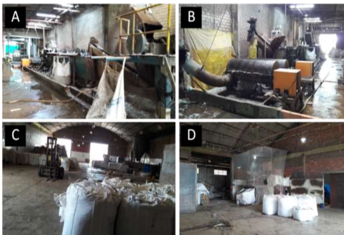
Figure 3: Plastic recycling process of the plant under study: (A) Plastic washing process, consisting of grinding mill and washing tank; (B) Process of centrifuging the washed plastic; (C) Plastic storage tank; (D) and Plastic extrusion process.
