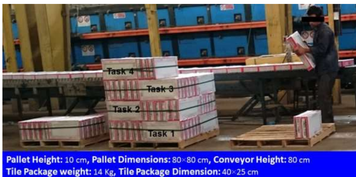
Figure 1: Loading tile packages, from conveyor to pallet
