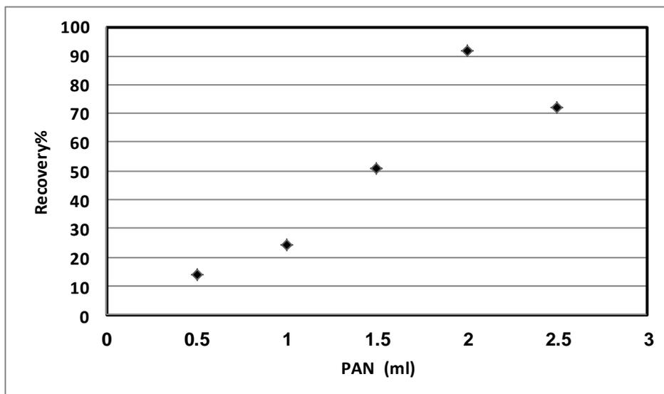
**Figure 1:** Effect of 1-(2-Pyridylazo)-2-naphthol (PAN) ligand rate on extracting Zn cation ( $Zn^{2+}$ ) by USAE-SFODME method. Extraction conditions included: 10 ml of urine sample, spiking  $0.8 \mu\text{gml}^{-1}$  of standard  $Zn^{2+}$ ,  $90 \mu\text{l}$  of 1-dodecanol, pH = 5.5, temperature =  $35^\circ\text{C}$ , sonication time = 20 minutes.
