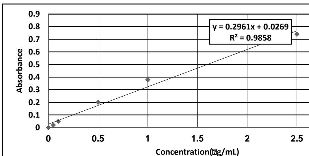
**Figure 6:** Calibration curve and linear equation for zinc standards with concentrations 0.05, 0.10, 0.50, 1.00 and 2.50  $\mu\text{gml}^{-1}$ . The correlation coefficient of  $r = 0.99$  indicates appropriate conditions for the standard rates regarding zinc analyte
