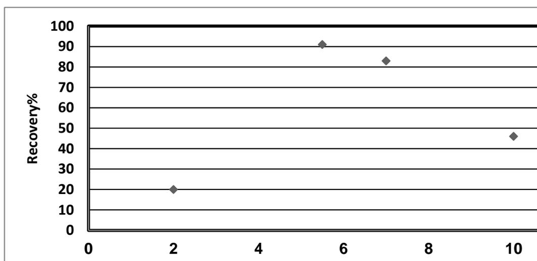
**Figure 2:** Effect of pH on extracting Zn cation ( $Zn^{2+}$ ) by USAE-SFODM method. Extraction conditions included: 10 ml of urine sample, spiking  $0.8 \mu\text{gml}^{-1}$  of standard  $Zn^{2+}$ , 2 ml of 1-(2-Pyridylazo)-2-naphthol (PAN) ligand,  $90 \mu\text{l}$  1-dodecanol, temperature =  $35^\circ\text{C}$ , sonication time = 20 minutes.
