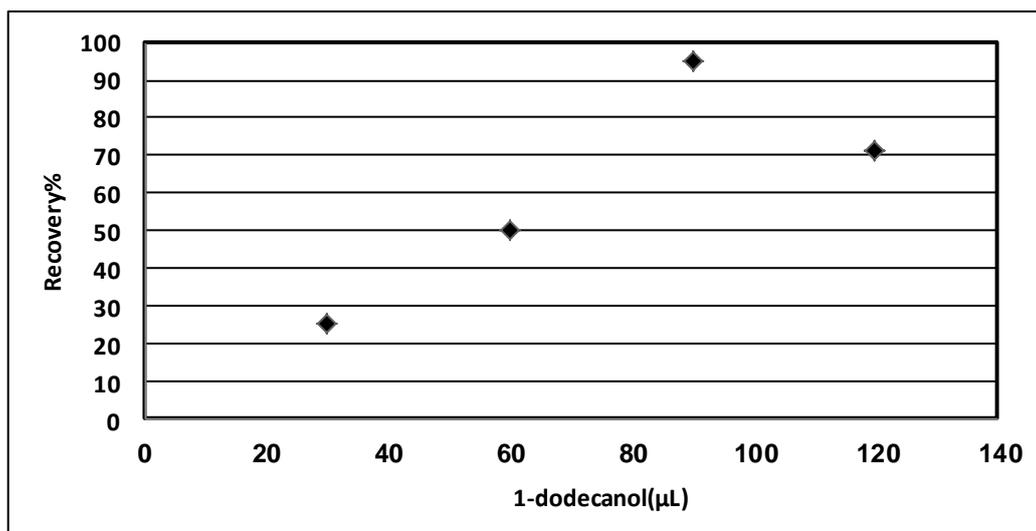
**Figure 5:** Effect of the amount of 1-dodecanol on extracting Zn cation ( $Zn^{2+}$ ) by the USAE-SFODME method. Extraction conditions included: 10 ml of urine sample, spiking  $0.8 \mu\text{gml}^{-1}$  of standard  $Zn^{2+}$ , 2 ml of 1-(2-Pyridylazo)-2-naphthol (PAN) ligand, pH = 5.5, sonication time = 25 minutes.
