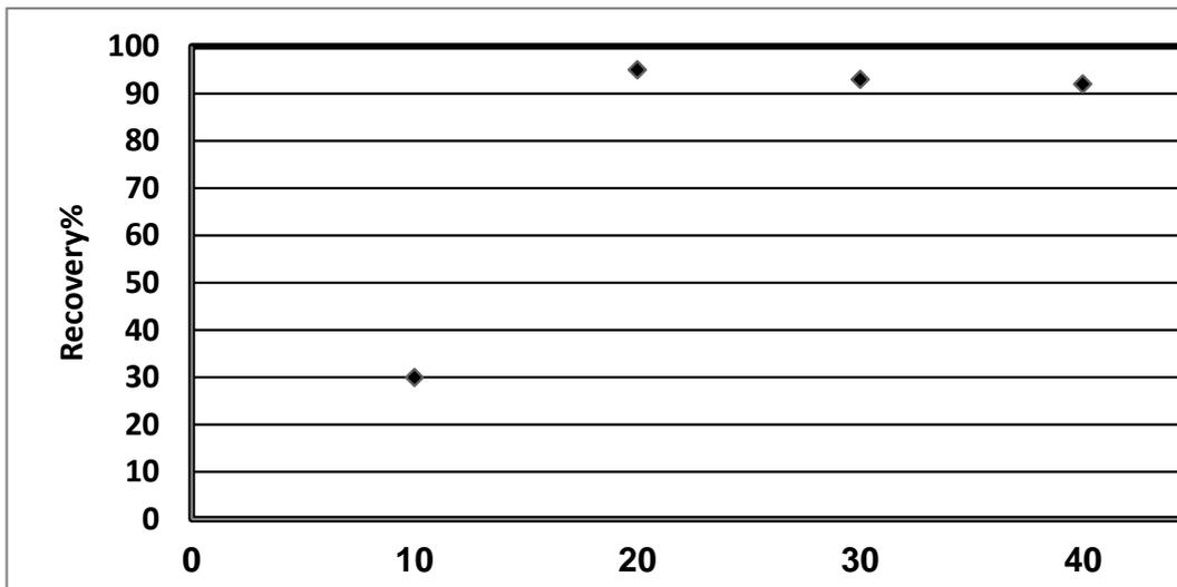
**Figure 3:** Effect of sonication time on extracting Zn cation ( $Zn^{2+}$ ) by USAE-SFODM method. Extraction conditions included: 10 ml of the urine sample, spiking  $0.8 \mu gml^{-1}$  of standard  $Zn^{2+}$ , 2 ml of 1-(2-Pyridylazo)-2-naphthol (PAN) ligand,  $90 \mu l$  1-dodecanol, pH = 5.5, temperature =  $35^\circ C$ .
