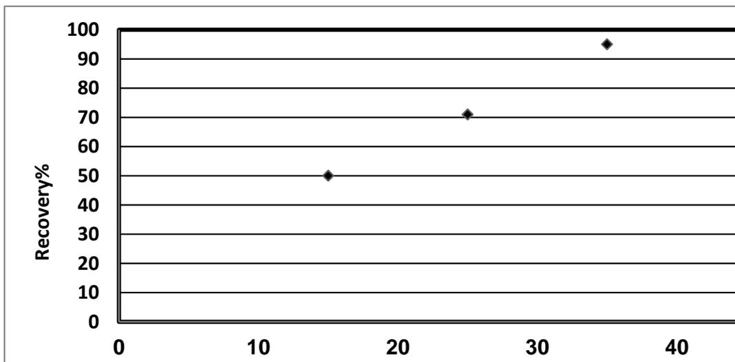
**Figure 4:** Effect of temperature on extracting Zn cation ( $Zn^{2+}$ ) by USAE-SFODME method. Extraction conditions included: 10 ml of urine sample, spiking  $0.8 \mu gml^{-1}$  of standard  $Zn^{2+}$ , 2 ml of 1-(2-Pyridylazo)-2-naphthol (PAN) ligand,  $90 \mu l$  1-dodecanol, pH = 5.5, sonication time = 25 minutes.
