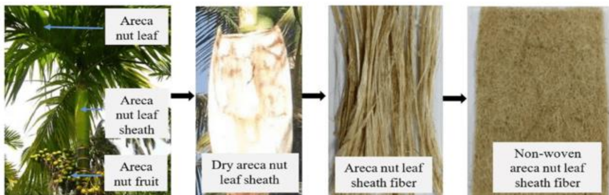
Fig 1. Areca nut palm leaf sheath fibers used for simulation in this study [27].
