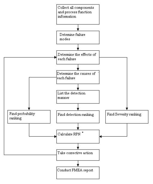
Figure 1: Failure mode and effects analysis (FMEA) process (6)
